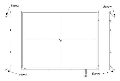
Figure 4-72 Replacing Samsung fluorescent lamp (WXGA) (3)
